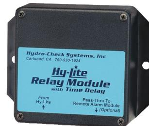
The Relay Module allows the Hy-Lite to perform as a controller of valves, custom alarm systems, etc. A 1 amp SPDT relay features an adjustable time delay to compensate for expected equipment rinse-up times. There is also a signal pass-thru feature permitting the relay module to be used with the remote alarm module.
