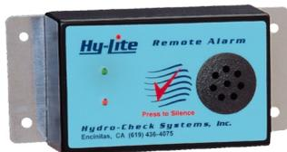
The Remote Alarm Module has a peizo alarm, green/red LEDs, and silence switch to duplicate the operational status of the connected Hy-Lite. Both units act as a system, since silencing the alarm at either location will silence both alarms. The alarm module can also be ordered with an auto re-alarm feature.
