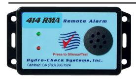
For an audible alarm at the monitor-controller or audible & visual indication at a separate location, the 414RMA features green/flashing red LEDs and peizo alarm. The system may be connected to any of the 414 Monitor/Controller models as well as controllers of other manufacture that feature a dry-contact setpoint relay. Installation can be at distances up to 700ft.
