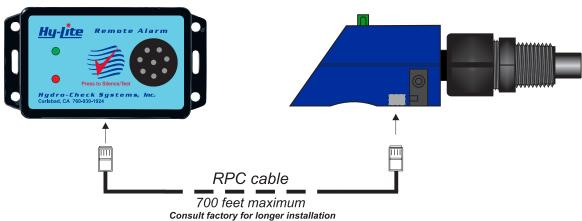
1) Once a suitable location has been found, attach the Remote Alarm Module using the screws provided, or screws suited to the material. 2) Connect the interconnecting RPC cable to the module and Hy-Lite as shown. The Hy-Lite powers and signals the remote, no other connections are necessary.
