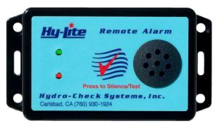
The Remote Alarm Module can be installed at distances *up to 700 feet!* Both module input and Hy-Lite output ports utilize telephone "handset" connectors for fast and easy, *click-click*, installation. Cables are available in standard 10, 50, 100 & 200 ft lengths. Custom lengths can be ordered, or quickly fabricated on-site with the aid of an appropriate crimping tool.
